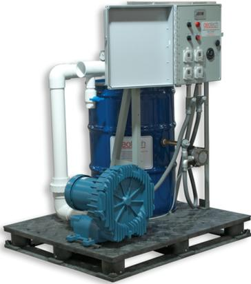
Designed to remove hazardous vapors from the subsurface by drawing air through contaminated soil, and volatilizing adsorbed phase pollutants. Ideal for well point or trench type vapor barriers. These systems are factory assembled and fully tested for function, performance and safety to meet the design conditions of each site application.
